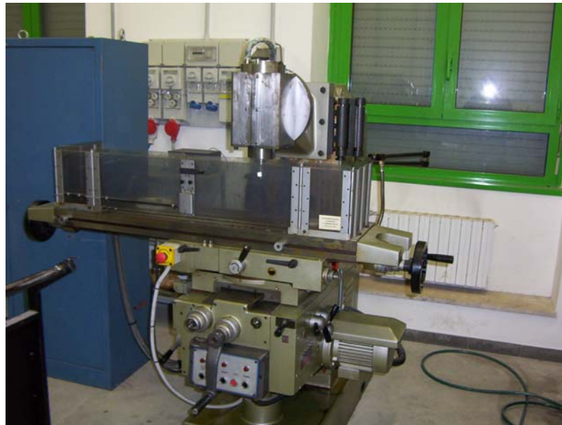
Fig.5 Universal milling used for the drilling operations
