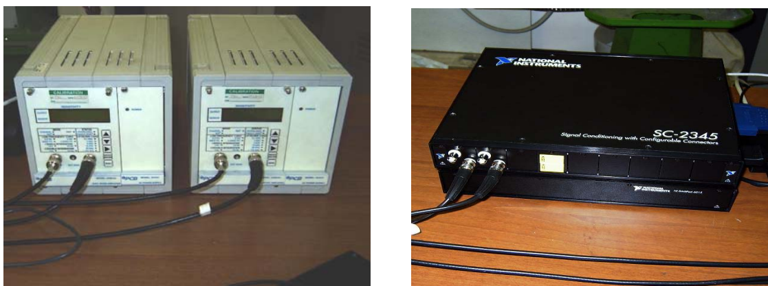
Fig.7 Amplifiers type PCB 443 B102 and acquisition schedule type N. I. SC-2345 N
