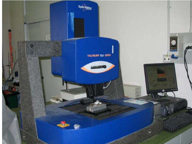
Fig.10 Instrumentation used to roughness measurements on the hole surface
