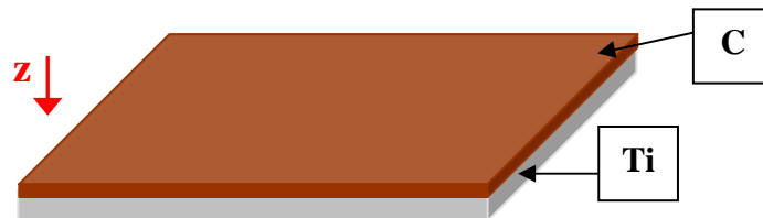
Fig.7 Sketch of the prepared sample to a better physical simulation for diffusion phenomena with the z direction for the XPS profile observation
