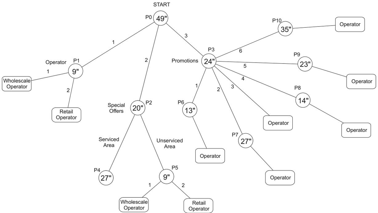
**Fig. 5.** Example of an IVR system in a call center. In each node we show the average time (in seconds) that a given user spends listening to option messages. Also, in each link we show the number of key that the user must press in order to advance to the required service.
