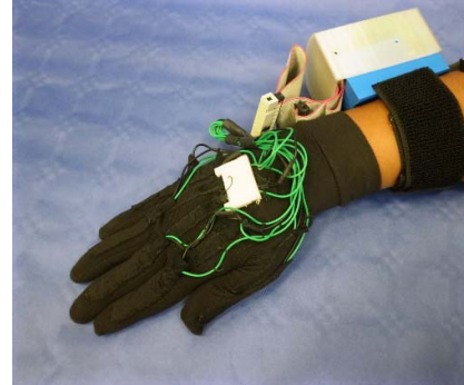
Fig.2. The two sensory unit. The dataglove for the IP and MP hand joints.
