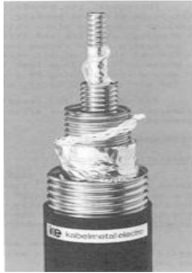
Figure 110: A cross section of a flexible transfer line developed at CERN in collaboration with Kabel Metaelectro [330]
