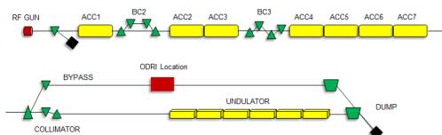
Figure 3: Layout of FLASH linac (not to scale). The location of the ODRI experiment on the bypass line is indicated.
