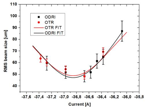
Figure 5: Quadrupole scan results. The beam sizes (rms) determined from ODRI angular distribution (black) and from OTR images (red) are shown as a function of the quadrupole current.
