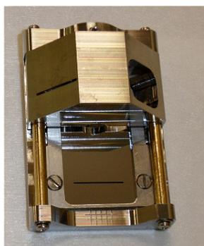
Figure 2: Photo of the target holder. The electron beam enters from left, and the produced radiation leaves the screen from the hole on the right. The first slit can be moved by a stepper motor into different vertical positions. A calibration pattern is visible in the bottom part of the holder.
