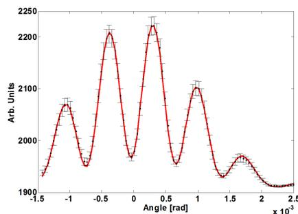
Figure 4: Example of a measured central profile of an ODRI angular distribution. The fit calculated by Minuit is superimposed (red line). The cut on the left of the angular distribution is due to a stray light reaching the camera.
