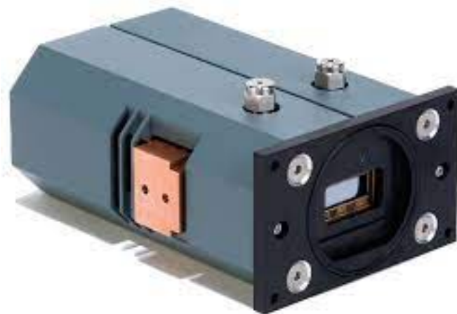
Figure 15. Andor DX 420 BR-DD for X-ray detection.
