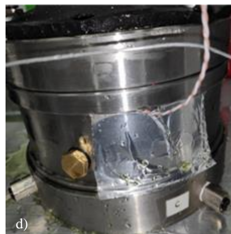
Figure 1. Experimental apparatus: (a) original oedometric cell; (b) thermostatic bath; (c) insulation system; (d) thermocouple.
