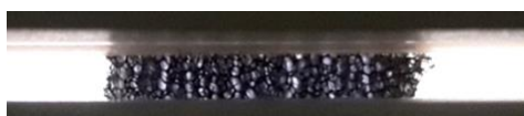
Figure 1. Photograph of the DBD during the plasma treatment of a PU foam
