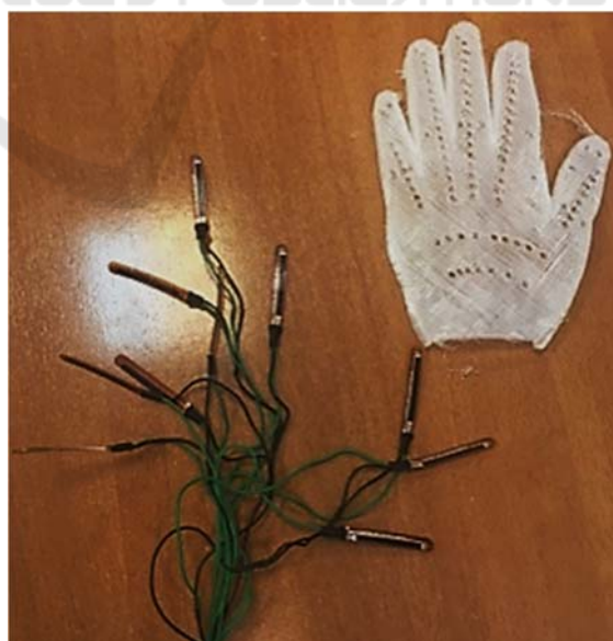
Figure 2: Flex sensors' wiring (left down) and 3D printed prototype (right up).
