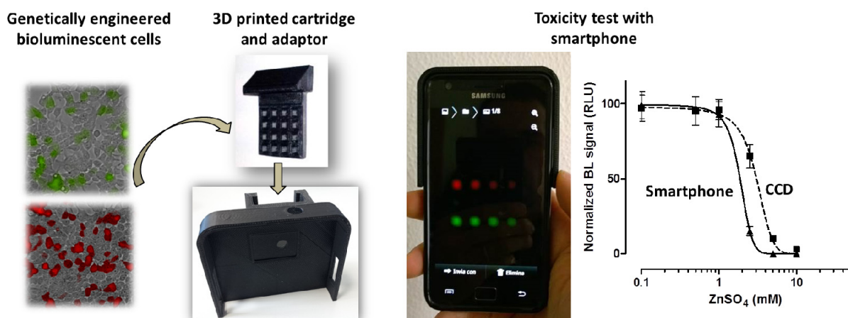
Figure 1. Overview of the SMART (CELL) 2 PHONE device. Genetically engineered BL mammalian cells (SMART CELL) were integrated into 3D printed cartridges and exploited as toxicity biosensor using a CELL PHONE as detector.
