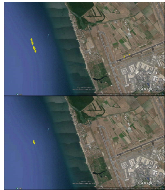
Figure 11- Comparison of a ADS-B track, free and jammed channel
