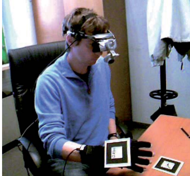
Fig. 10.8 An example of integration between a pattern-based tracking system and a data glove for hand position and gesture acquisition in an augmented reality environment
