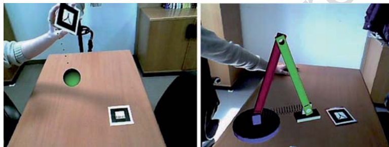
Fig. 10.4 Marker-based tracking for implementing interactive AR simulation of dynamic systems: launching a bouncing ball (on the left ) and moving a slider-crank mechanism with a spring damper element
