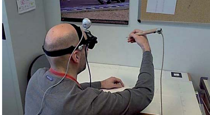
Fig. 10.5 Magnetic device-based tracking for implementing interactive AR geometric modeling environment
