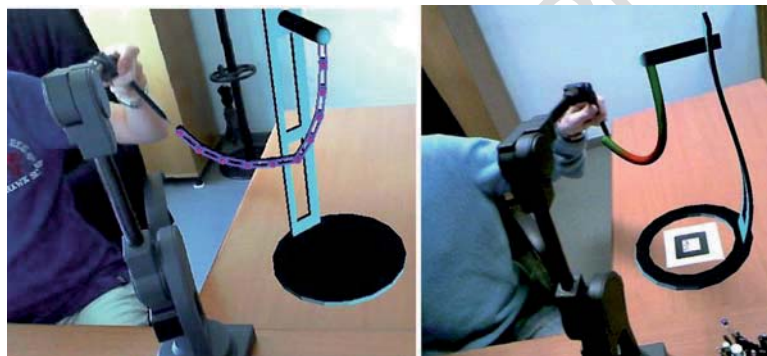
Fig. 10.7 Mechanical device-based tracking for implementing interactive AR engineering simulation of motion: ten pendula simulation (on the left ) and flexible slender beam (on the right )
