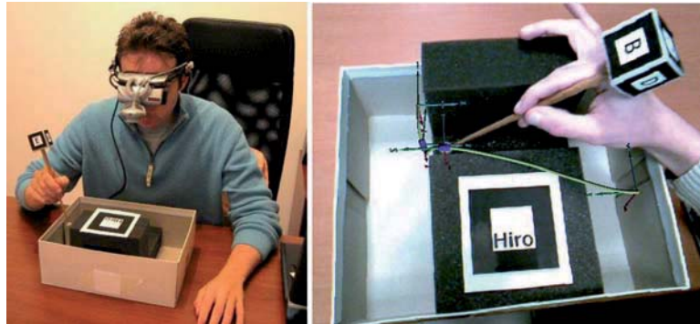
Fig. 10.3 Marker-based tracking for implementing an interactive AR procedure for supporting cable harnessing
