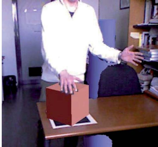
Fig. 10.11 Occlusion management using depth map acquisition and computation
