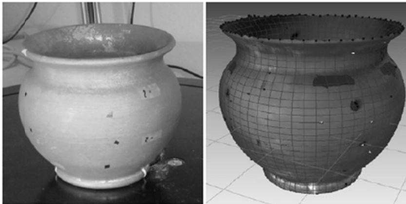
Figure 2. An example of a real vase (on the left) and its virtual replica built from a laser scanner acquisition (on the right).
