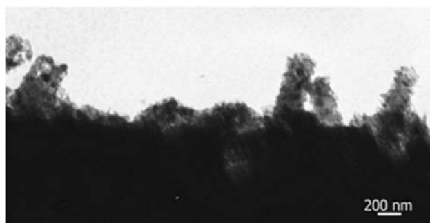
FIGURE 6: TEM image of a polyaniline-nanodiamond film composite
