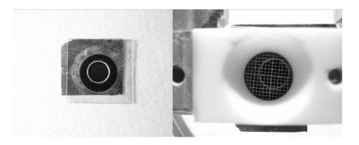
**FIG. 3:** Left: a CNTs sample and a mica spacer (with a 4 mm central hole) on it. Right: the MACOR holder keeps together the grid, the mica spacer and the CNTs sample.
