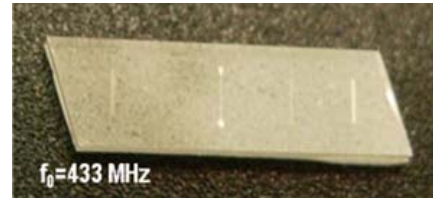
Figure 13. Photo of the SAW ID-Tag operating at 433.92 MHz.
