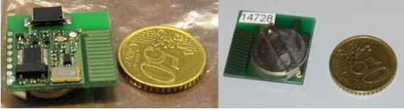
Fig. 5. The Active Tag Board with the 2.65 GHz antenna (upper side) and 433 MHz printed coil antenna (right side). (Courtesy of AME Srl)
