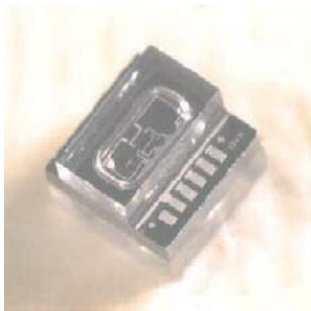
Fig. 1.7 Silicon pressure sensor SP15 bonded with glass cover (courtesy by SensoNor AS An Infineon Technologies Company).
