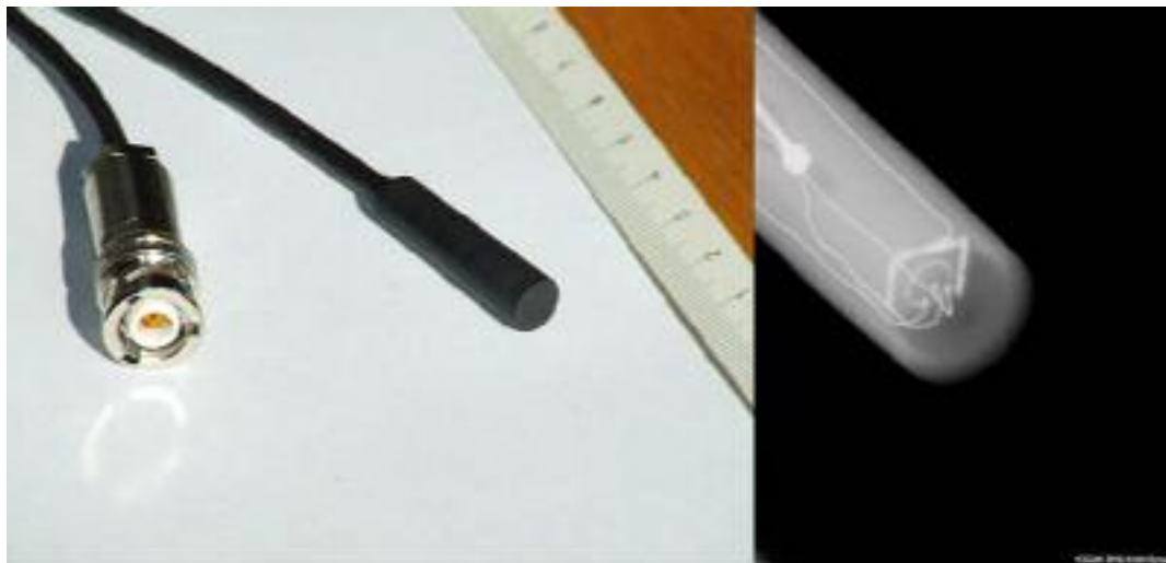
Fig. 5.4.a) Image of the CVD dosimeter with the connection cable and the PMMA housing painted with graphite-based lacquer. b) X-ray image of the CVD dosimeter. It is possible to identify the squared diamond element, the signal cables, and the circular aluminium dot on the top of the intrinsic diamond layer.
