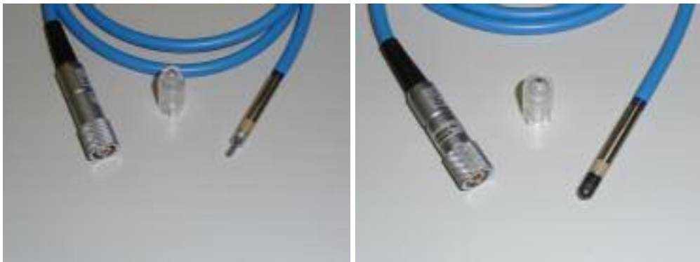
Fig. 5.17 The two commercial Ionization Chambers used for testing the performances of the Single Crystal Diamon Dosimeter; PTW type 31014 Pin Point Chamber (on the left) and PTW type 31010 Semiflex Chamber (on the right).
