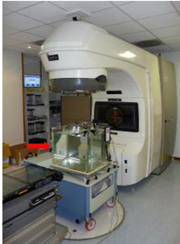
Fig. 5.7. The CLINAX DHX Accelerator with the PTW motorized water phantom MP3 (red arrow)
