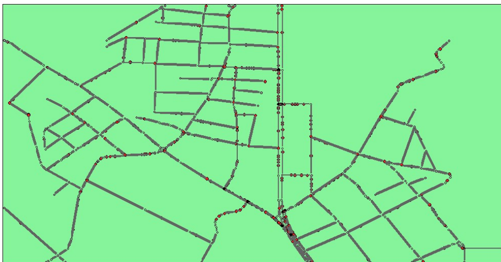
Figure 4.7: Vanetmobisim road topology example imported from OpenStreetMap database. The map showed in this picture ("Quarto Miglio" district in Rome) was exported in xml-format from OpenStreetMap and then imported into Vanetmobisim simulator. The red dots represent the constrained vehicles moving to across roadmap during the simulation.
