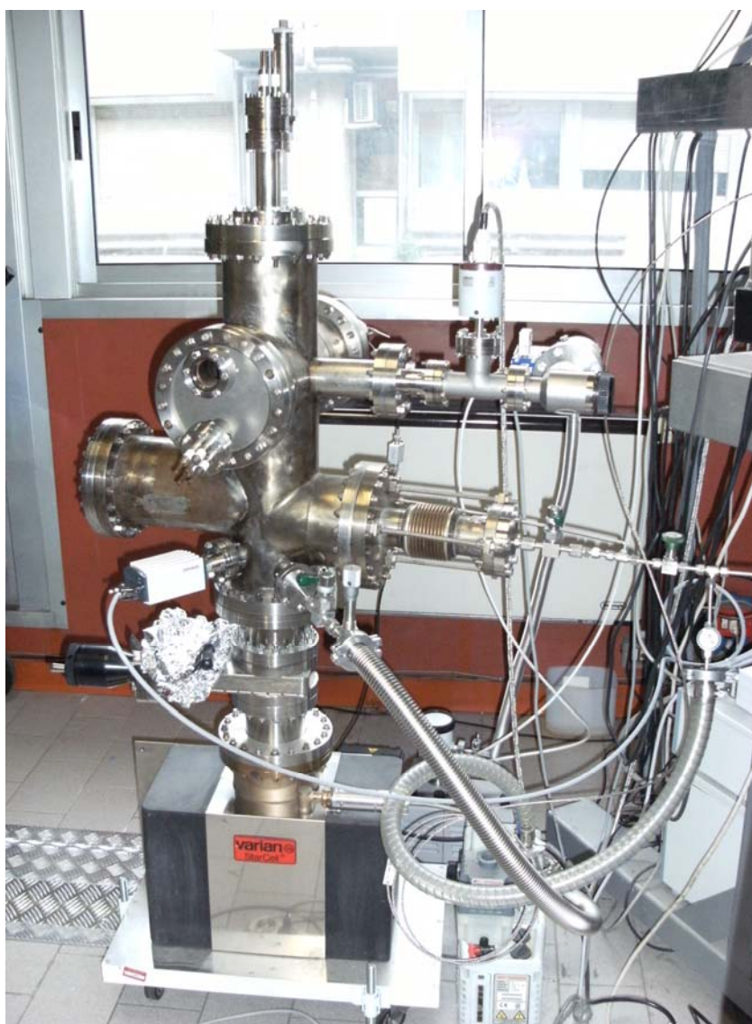
Fig. 9. Picture of the CVD chamber at the Dept. of Physics, University of Rome “Tor Vergata”
