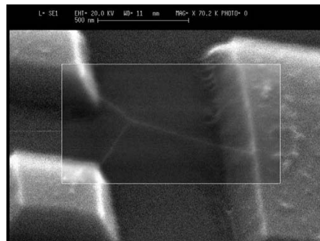
Fig. 30. Best results of MWCNTs selective deposition for transport measurements. The density of MWCNTs is low (a) and many of them connect neighbouring mesa (b) and (c).
