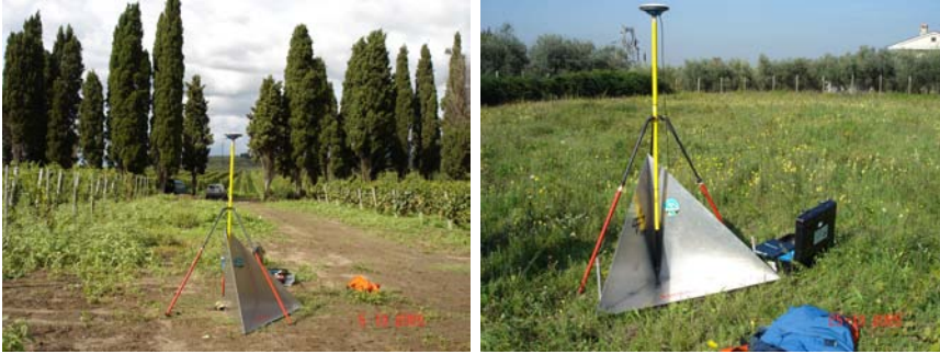
Figure 3.3: The corner reflector for radiometric calibration. It is possible to notice also the GPS equipment for the geocoding operation.
