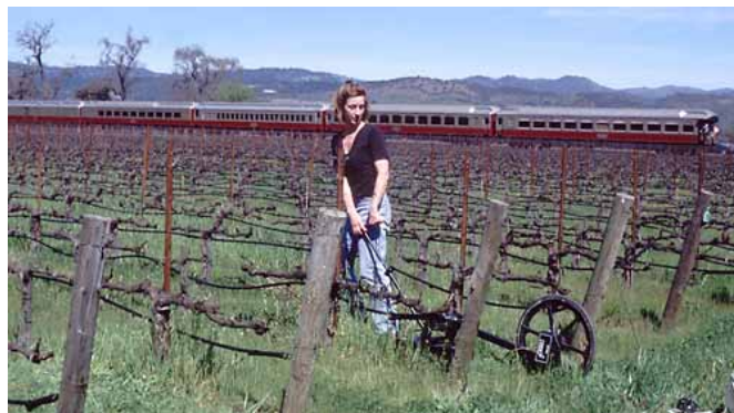
Figure 1.17: Ground Penetrating Radar (GPR), (Rubin et al., 2002).
