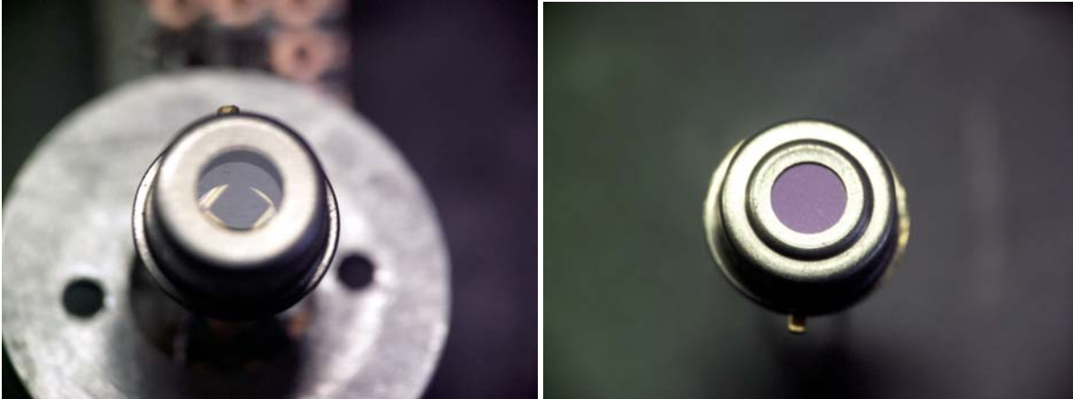
a. b. Figure 3: Detail thermopiles: a Call sensor b. Melexis
