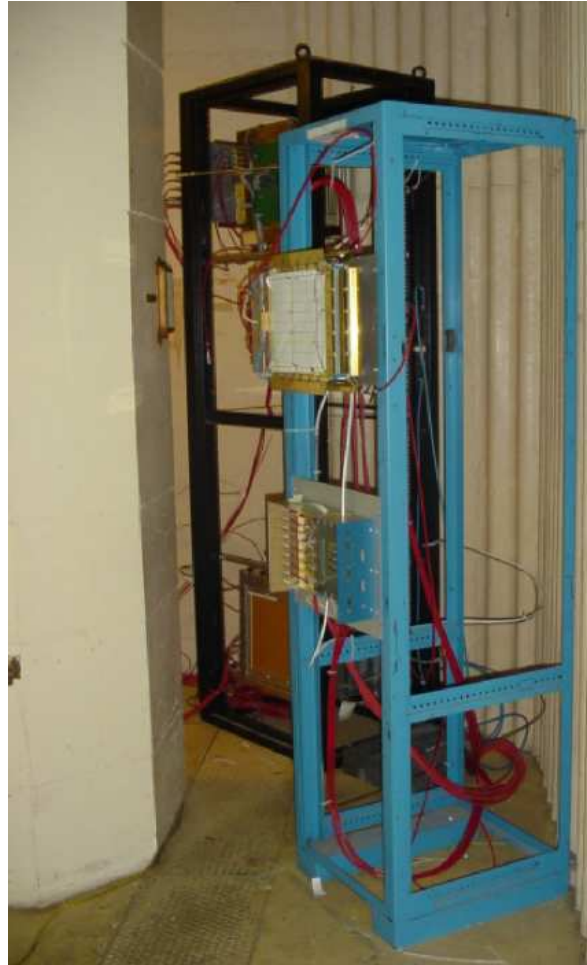
Figure 4.47: Position of the chamber during the test. On top of the blue rack was placed the chamber A and B. On the black rack, where the radiation flux was less intense, was placed the chamber C.
