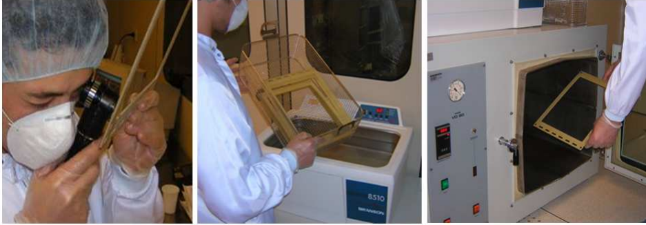
Figure 4.18: The clean procedure of the frame. From the left to the right: the visual inspection; the cleaning in the ultrasonic bath; the drying in the oven at 80 °C.
