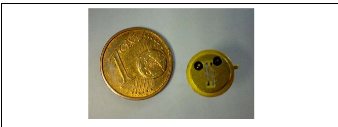
Fig. 33: transduction element for DMMP detection.
