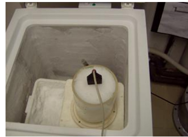
Fig. 5. TDR probe in snow-filled mould
