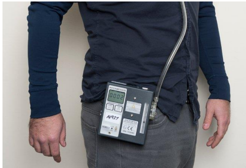
(Figure.22. Chemical Exposure Monitoring device in Food (Horlicks) Industry)
