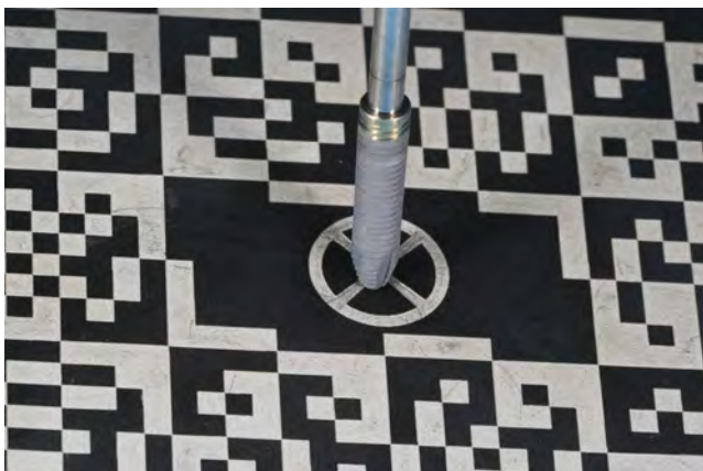
FIGURE 5 Calibration of implant length on the calibration plate
