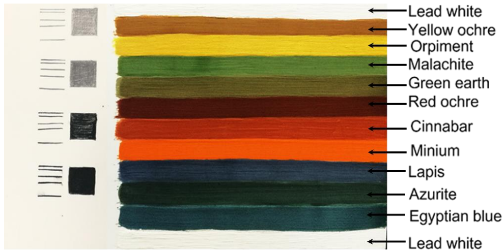
Figure 3.4 - Wooden sample: colour layer with different inorganic pigments.
