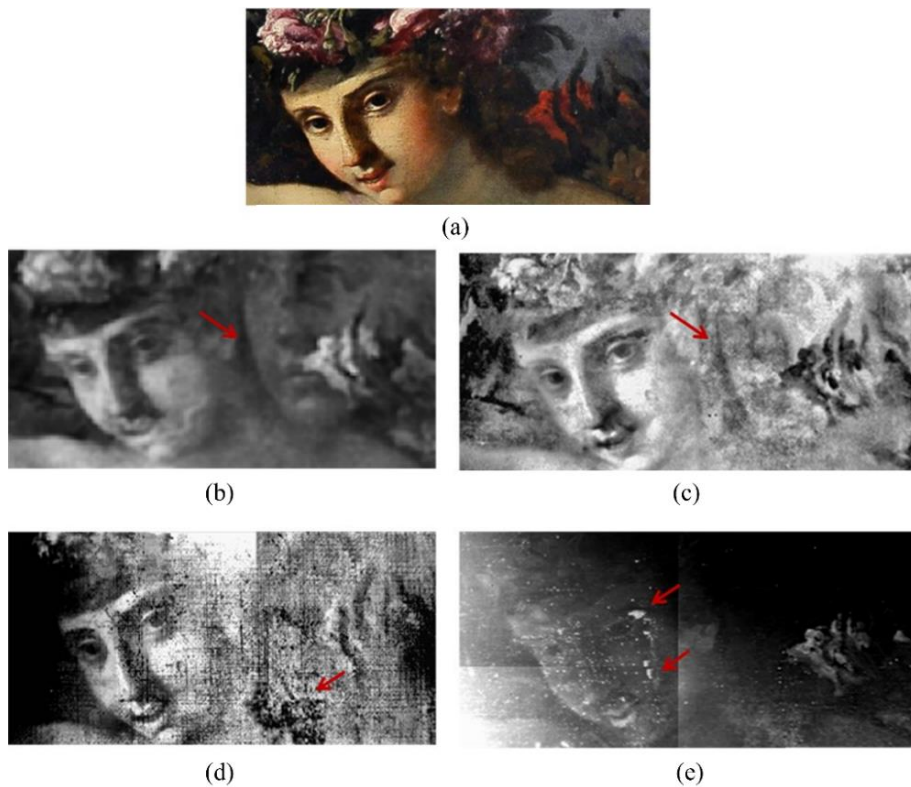
Figure 4.13 – (a) Detail of Figure 4.10; (b) IR-ITR image where another face is revealed; (c) thermogram recorded after 20ms to the light pulse where the arrow indicates the second face slightly visible; (d) thermogram recorded after 300ms to the light pulse where the canvas patten can be seen; (e) MWIR reflectogram where the arrows point at repaired lacunas.
