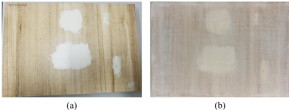
Figure 3.2 - Wooden sample: (a) large defects filled with ready-to-use plaster; (b) surface of the support finished with the gypsum preparation.
