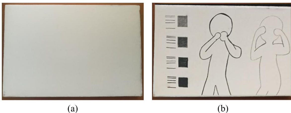
Figure 3.3 – Wooden sample: a) ground layer; b) underdrawings made by charcoal (left figure) and graphite (right figure). Black stripes and squares on the left were made (from top to bottom) with one and two layers of graphite and charcoal, respectively.
