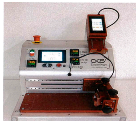
Figure 3. (left) Slot-die schematic process; (right) table-top coater with slot-die head.
