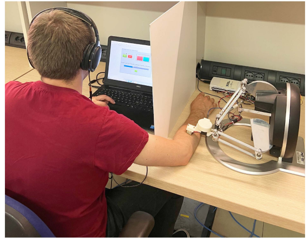
Fig. 1. Participant is using the graphical user interface to tune the temperature of the end-effector while his right forearm is stimulated. To avoid biases in the stimuli evaluation, the participant wears a headset providing white noise, and the cardboard panel prevents him from seeing his forearm during the stimulation.
