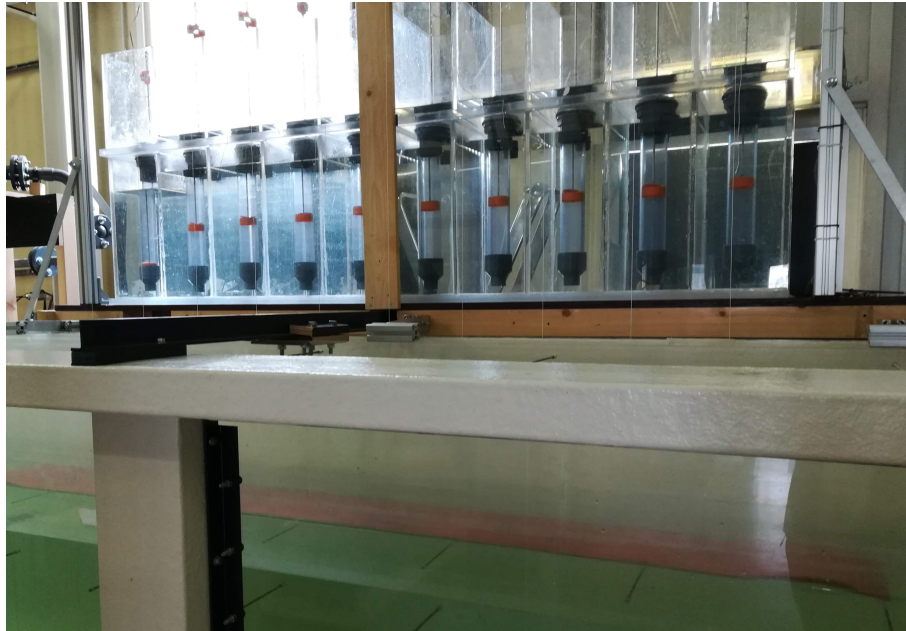
Figure 8. Laboratory model of the MP 2 PTO system, made by 10 pistons.
