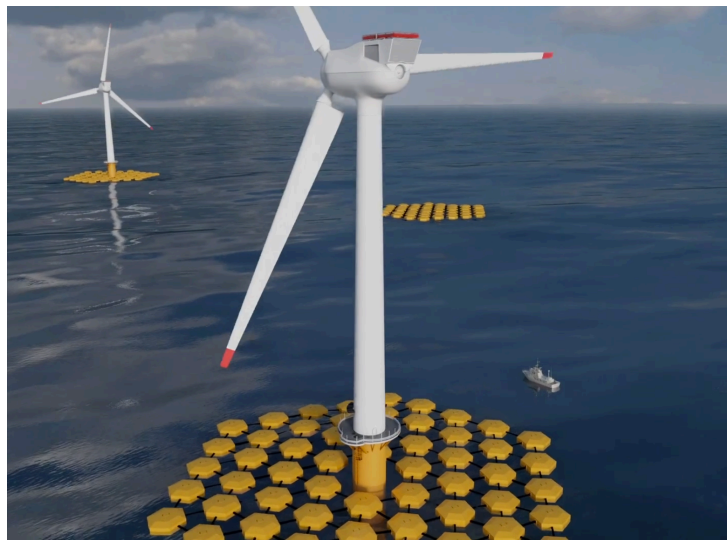
Figure 1. Artist’s sketch of a system of floater blanket wave energy converters (WECs) connected to offshore wind turbines. Source: www.oceangrazer.com .
