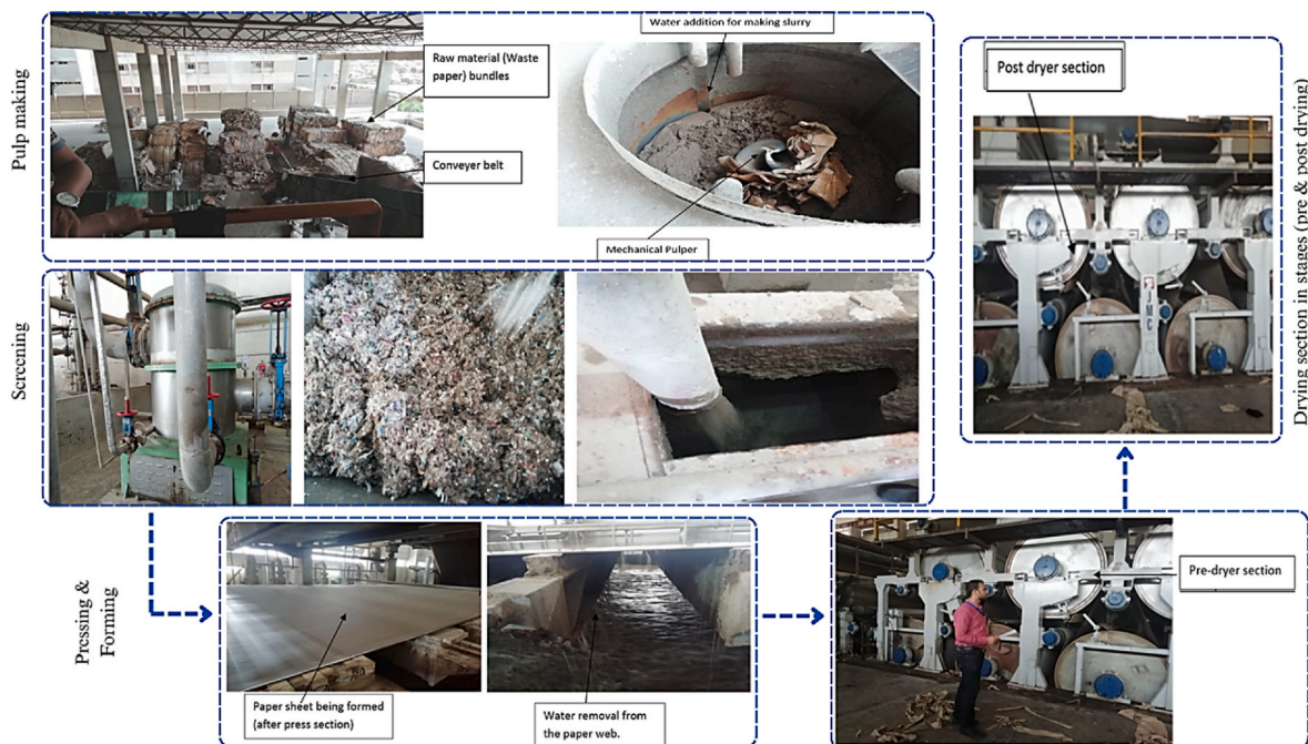
Fig. 8. Process flow of recycled paper manufacturing at an industrial facility.
