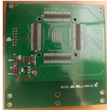
Fig. 6. Test board, back side. The BJT transistor for internal voltage regulation is highlighted by the red circle.
