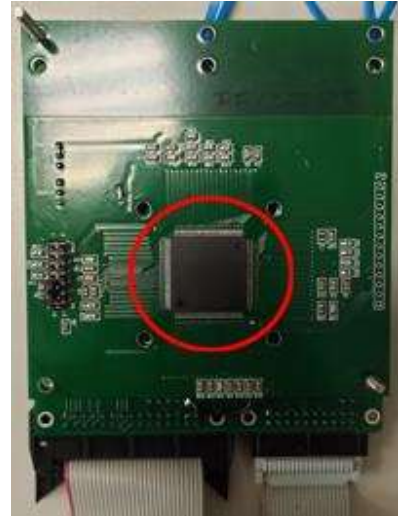
Fig. 5. Test board, front side. The DUT is highlighted by the red circle and is powered up by the control board via IDC connectors
