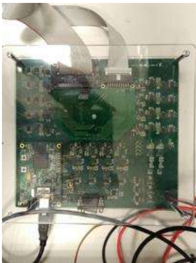
Fig. 4. Control board. The IDC connectors on top bring the power supply to the test board. The USB connector at the bottom gives access to the acquisition
