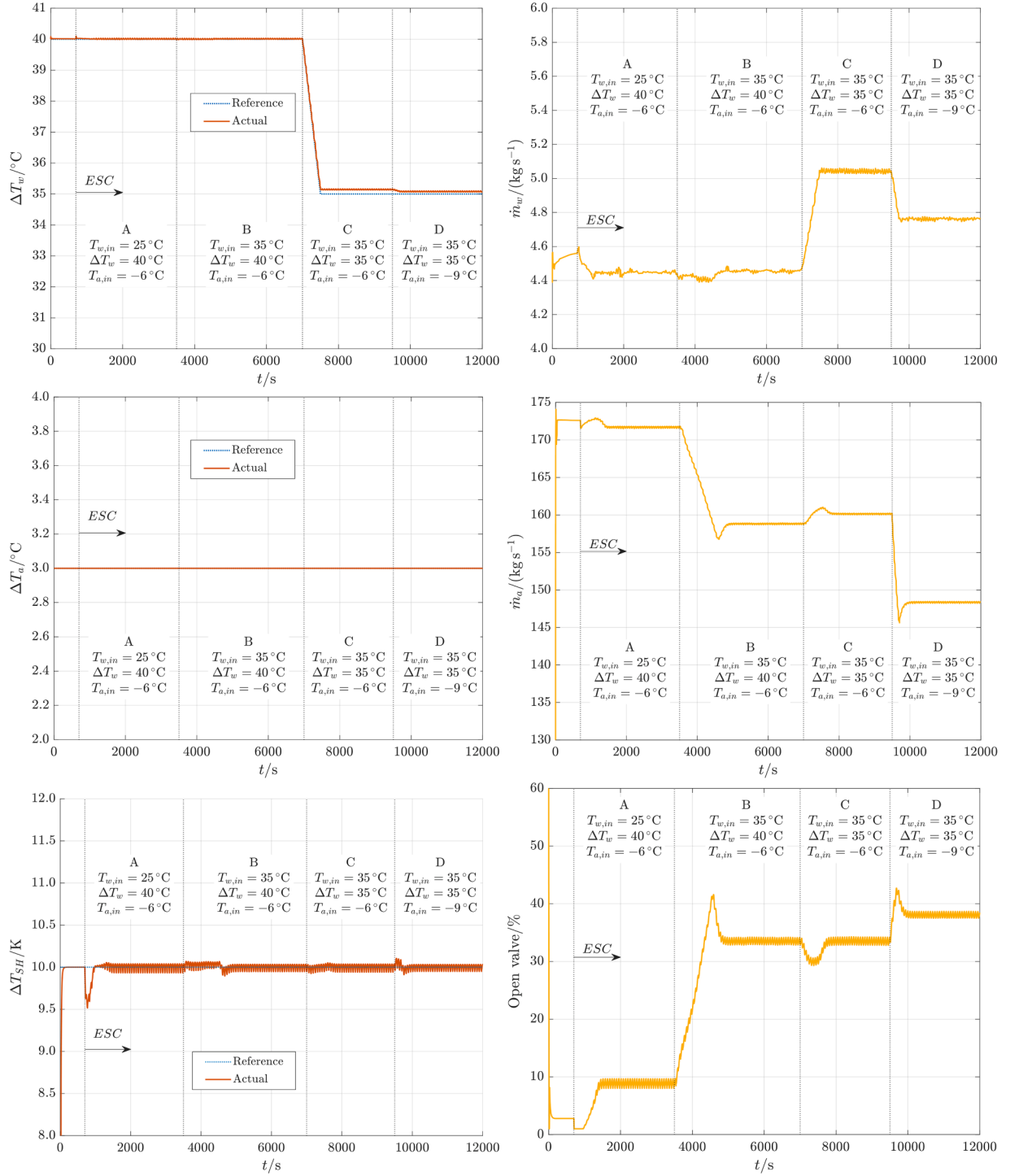
Fig. 9. Dynamic simulation results of the PI controllers: water temperature difference and mass flow rate (top); air temperature difference and mass flow rate (middle); superheat degree and bypass valve opening (bottom).
