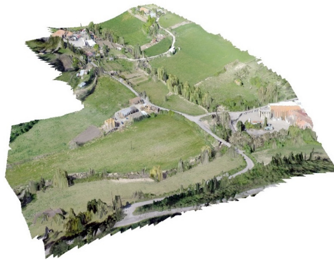
Figure 3. 3D scene of the Drone-derived Digital Surface Model (DSM) and orthophoto.
