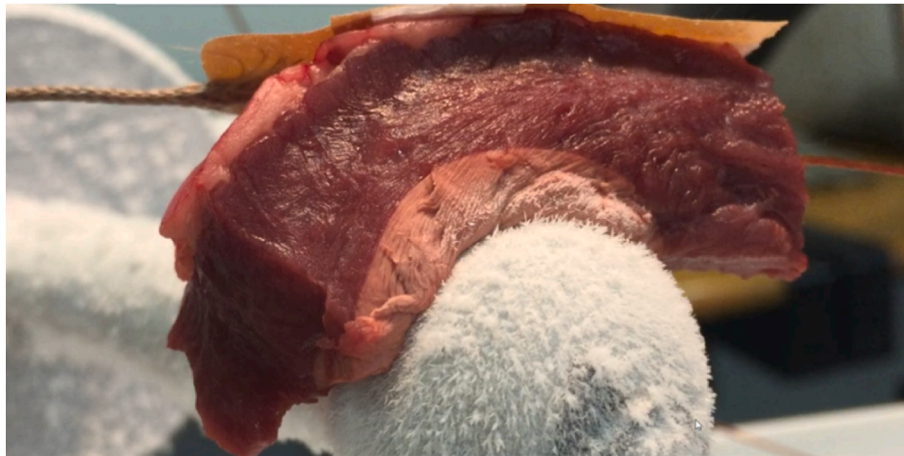
Fig. 3. Photo of a cardiac muscle piece placed on the cold finger after 20 s, clearly showing the ice front.
