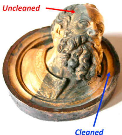
Fig. 1. Traditional PGAA spectra (left, arbitrary units) from two different regions of the bronze artefact (right) from the Baptistery of Florence. In particular, the uncleaned region (red) and the one cleaned using the Rochelle salts (blue) are shown. Data are adapted from Ref. [15]. In particular, the prompt-gamma lines from ^{35}\text{Cl} at 788.428 keV and 517.073 keV, discussed later, are marked with red arrows. Also, the prompt \gamma -rays from Ge isotopes [25], discussed in Sec. 2.3, are reported as green pulses with intensities in units of 10^{-2} b. (For interpretation of the references to colour in this figure legend, the reader is referred to the Web version of this article.)
