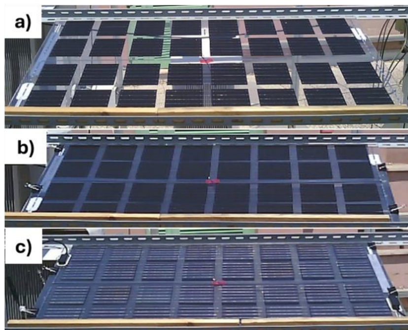
Figure 17 – Acquisition of I-V curves for bifacial (a), monofacial front (b) and monofacial rear (c) configurations.
