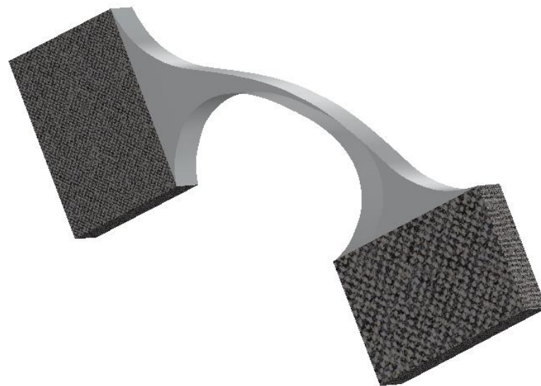
Figure 1. Connection of two rigid bodies through a flexure-hinge.
