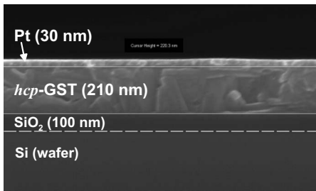
FIG. 1. SEM cross-sectional image obtained after the sample had been thermally characterized. After the 400 °C annealing temperature is reached, the GST crystalline phase is observed. It is also seen that the Pt layer thickness remains unchanged during the characterization.
