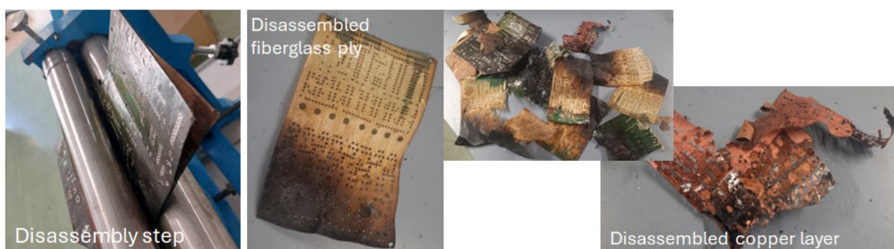
Fig. 5. Copper extraction from waste PCBs by thermo-mechanical disassembly.
