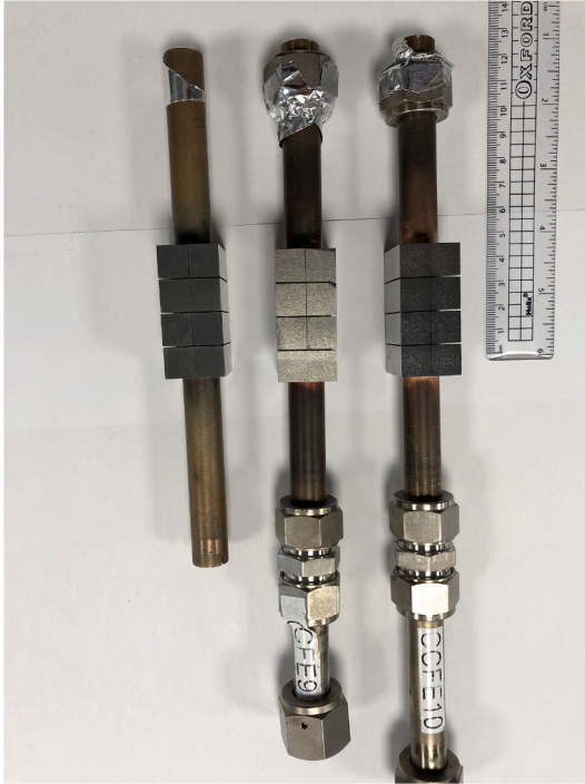
Fig. 2. Photograph of the phase 2 thermal break mock-ups specimens for the DEMO divertor target. From left to the right: as manufactured (CCFE11), with a single cycle at 25 \text{ MWm}^{-2} plus 100 cycles at 10 \text{ MWm}^{-2} (CCFE9), and before HHF testing (CCFE10).
