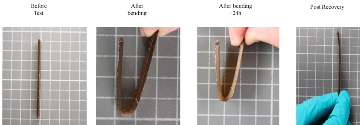
Figure 91: Shape Memory evaluation of 60PEEK-40PEI
