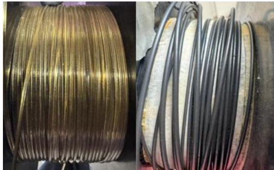
Figure 200: Produced filaments of blend (left) and composite (right)
