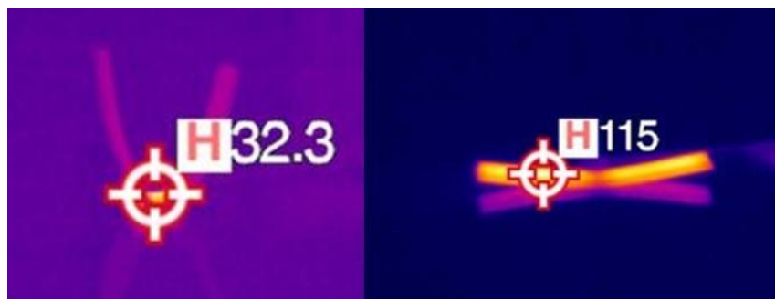
Figure 95: Thermal camera images of shape-memory recovery
