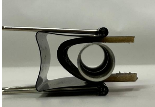
Figure 85: Sample forced to assume U-bent configuration
