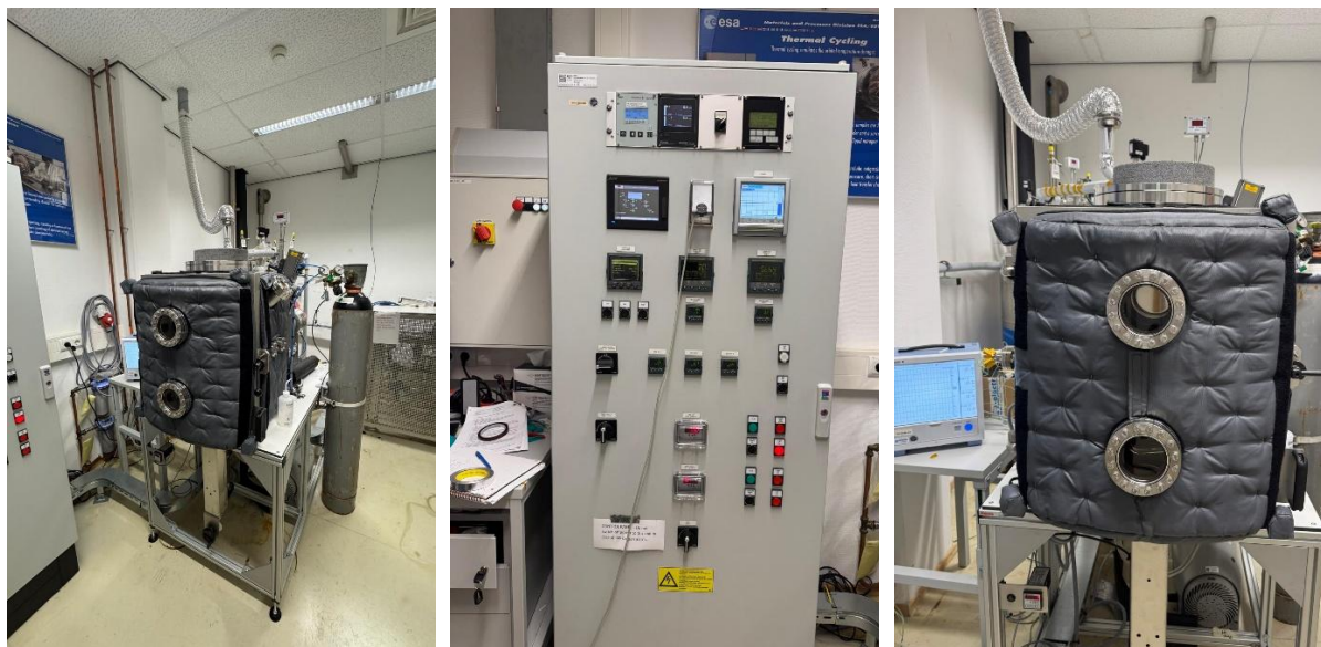
Figure 131: TVAC facilities in the ESTEC lab
