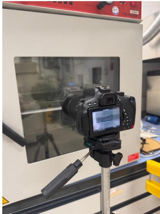
Figure 84: Shape Memory Test Set-up
