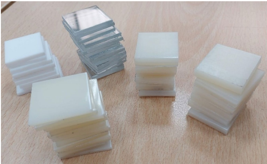
Fig. 1 Polymer samples treated with different abrasive papers and untreated ones
