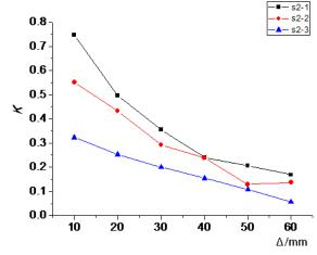
Figure 19. Stiffness degradation curve of S2
