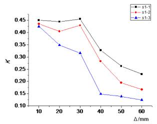
Figure 18. Stiffness degradation curve of S1
