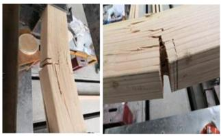
Figure 8. Midspan failure of S1 group
