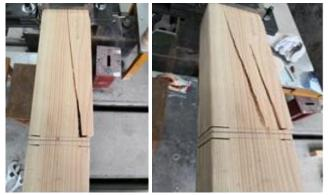
Figure 9. Midspan failure of S2 group
