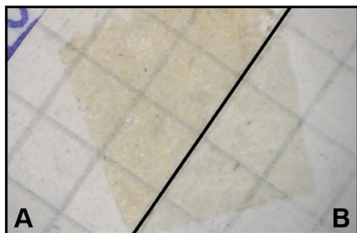
Fig. 8. Images of notebook sample with adhesive tape before (A) and after (B) cleaning with GGMA microgels.
