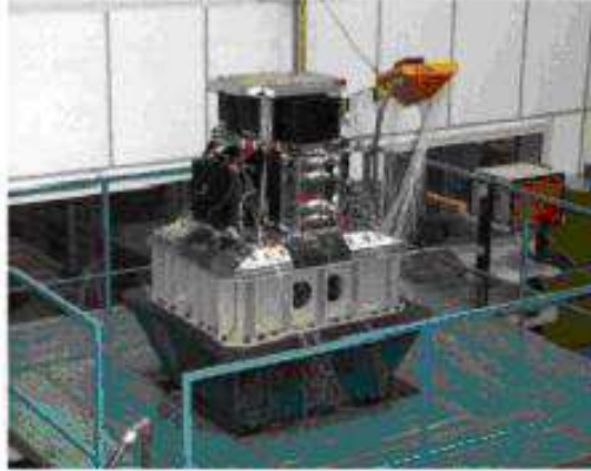
Figure 3.1: The PAMELA MDTM on the shaker system in IABG (August 2002).
