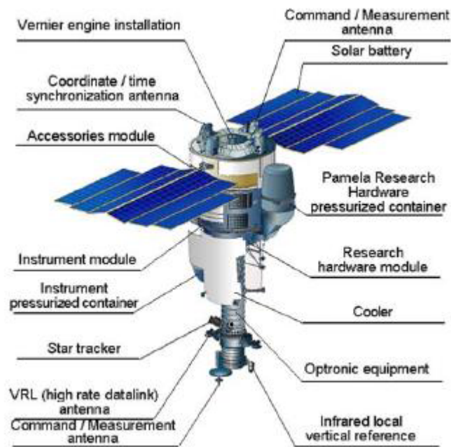
Figure 2.23: A sketch of the Resurs DK1 satellite which hosts the PAMELA experiment in a Pressurized Container. The satellite has a height of 7.4 m. The camera that will take high resolution images of the Earth is shown at the bottom of the figure. The shaded area on the right is the pressurised PAMELA container in data acquisition configuration. During launch and orbital manoeuvres, the container will be placed in the downward configuration.
