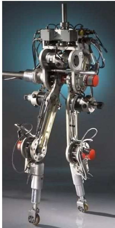
Figure 4.1: The five-link biped robot RABBIT.
