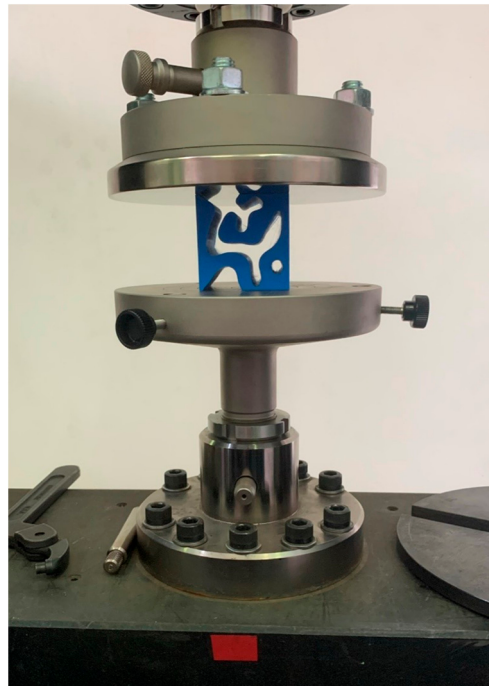
Figure 4. Experimental setup for metamaterial characterization.
