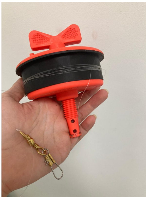
Figure 6.2. 4" PVC expansion well plug used to seal the head of the well and connection to the dosimeter with a nylon thread and a stainless steel carabiner.
