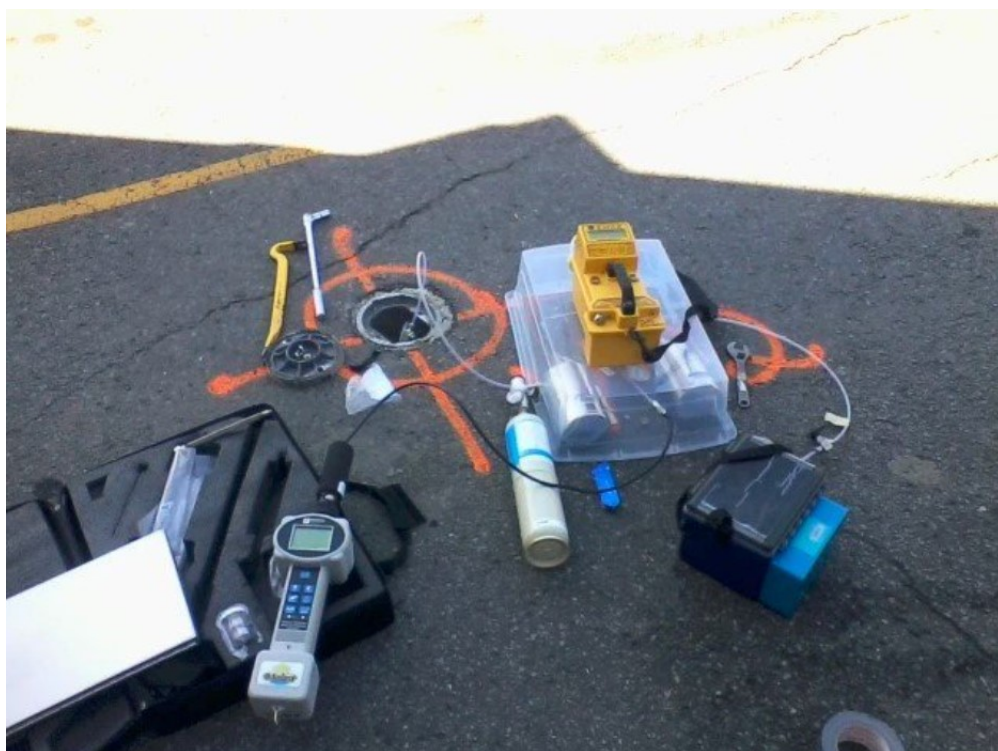
Figure 1.11. Active soil gas sampling using portable equipment (© ENVGUIDE)
